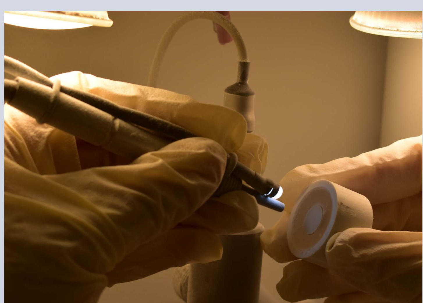
Figure 1, Sandblasting the PEEK disks with alumina; mean particle size of 50 \mu\text{m} and 110 \mu\text{m} .
