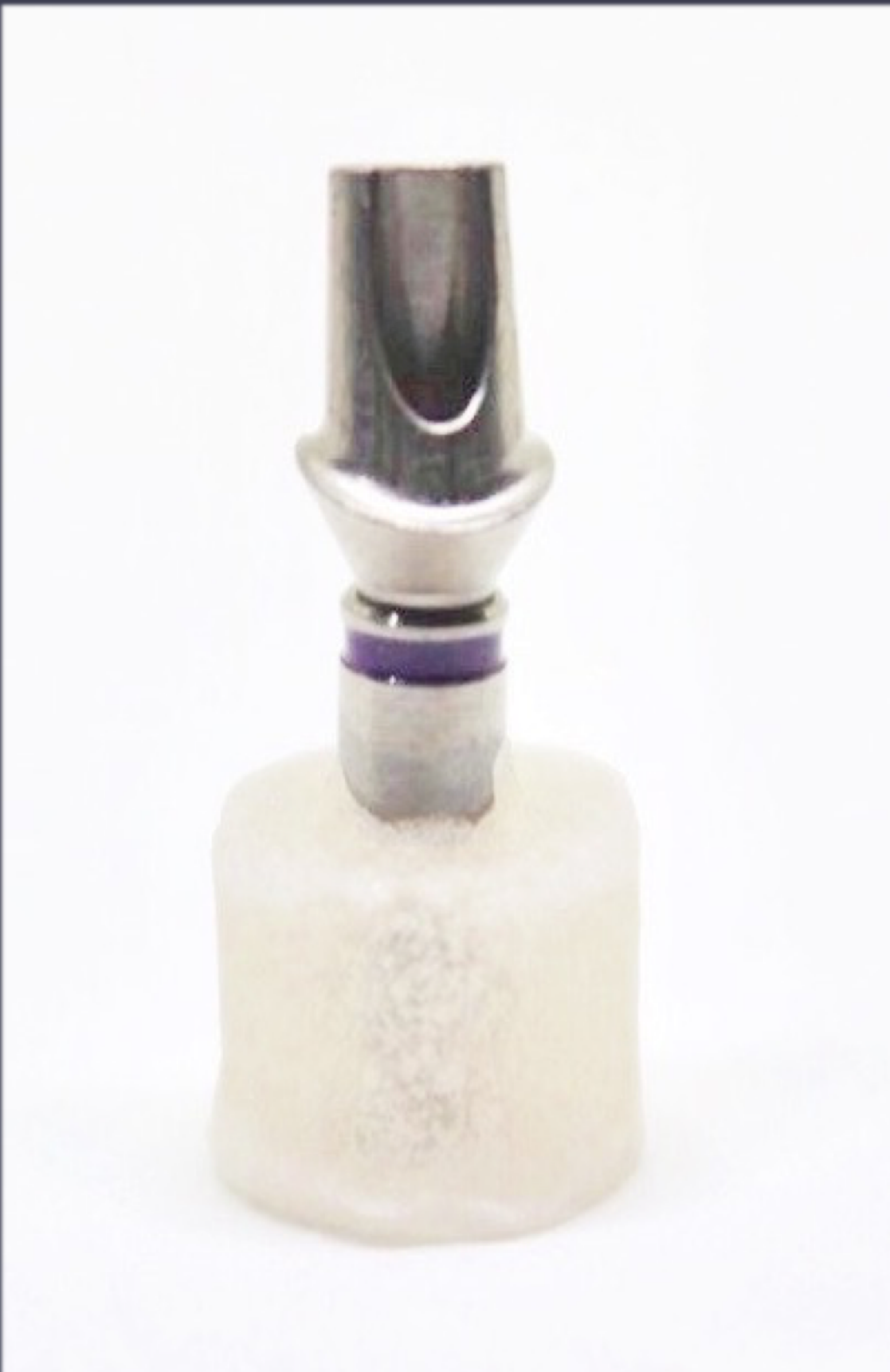
Fig 2: Ti implant abutment mounted on acrylic using surveying device.
